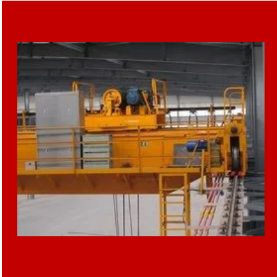
Double Girder Platform Cranes
